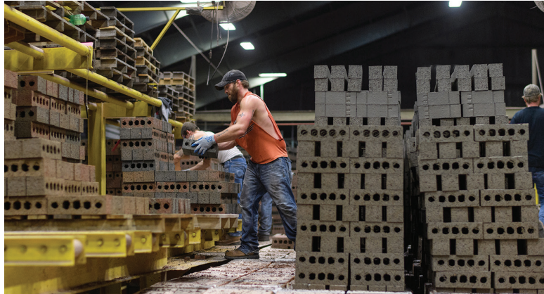
An employee unloads a kiln car and palletizes brick, which will later be sent to packaging.
